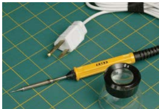
Fig. 2: Pencil-tip soldering iron and a loupe.
