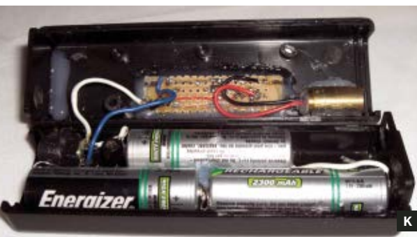
Fig. I: Laser diode wired in Digi-Key housing.
