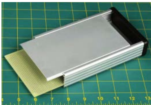
Fig. 4: Hammond Instruments project box and PCB.
