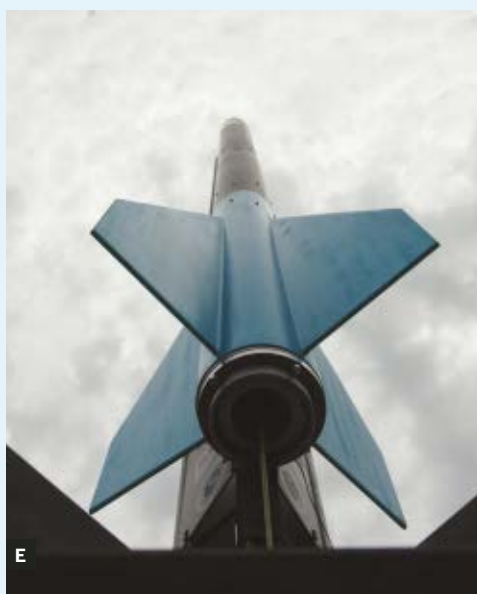
D. Composite fuel rocket engine installed and ready for liftoff. E. Carefully designed fins keep the rocket on course.
