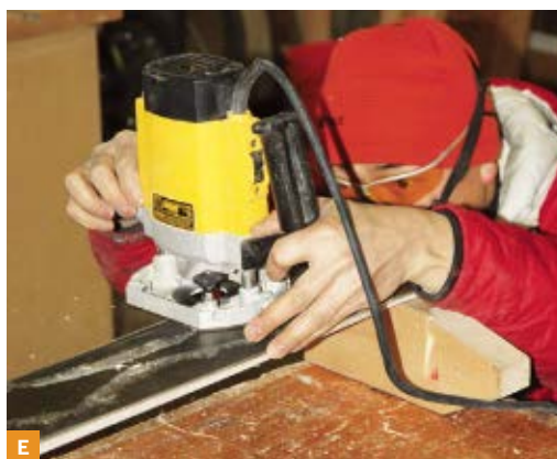
Fig. D: When they come off the press, the skis are attached to each other by the fiberglass sheet.
