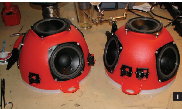
Fig. G: Speaker bolted in with washers and locking nuts. Fig. H: Terminal connected to the side of the bowl.
