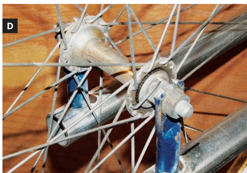
Fig. C: New fork legs tack-welded in place on either side of the original fork crown. Fig. D: Welding the dropouts to the fork legs.
