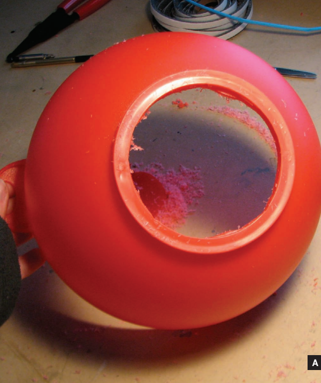
Fig. A: Hole cut in the bottom of the bowl. Fig. B: Template traced from hole piece. Fig. C: Side speaker position traced onto the bowl.
