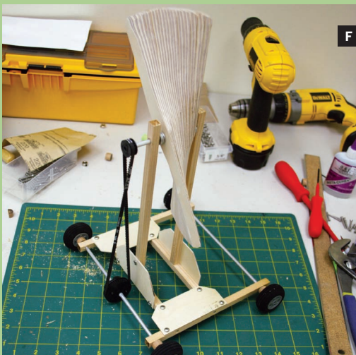
Fig. A: To make the propeller, cut 1"×10" strips of \frac{3}{32} " plywood, drill a center hole, and stack the strips on the \frac{3}{16} " aluminum rod, turning each one slightly before gluing it. Fig. B: The propeller completed, before sanding. Fig. C: The propeller profile after sanding. Fig. D: To join the sections of the frame, drill ample guide holes before driving in #4 screws. Fig. E: The frame completed, with plywood gussets. The uprights bend apart just enough to insert the propeller on its shaft. Holes for the shafts should be \frac{7}{32} " to allow them to turn freely. Fig. F: The completed cart, ready for testing. Plastic gears are attached to the shafts with cyanoacrylic glue. The wheels are a tight push-fit. The belt must be relatively loose to minimize shaft friction.
