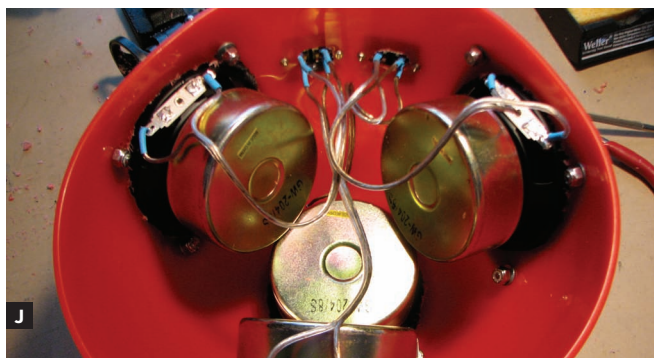
Fig. I: Two different terminal placement options: on opposite sides of the speaker, or together near the handle. Fig. J: Terminals connected, speakers all wired.
