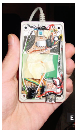
Fig. A: Bike-powered iPod charger detaches easily for parking. Fig. B: Original 6V hand-cranked charger with voltage stepped down to 5V for USB. Fig. C: Mouse case contains charger electronics and connects to bike dynamo via S-video plug on handlebars. Fig. D: iPod, opened-up charger, and iPod socks. Fig. E: Charger electronics, battery, voltage regulator, and USB port packed inside mouse case.
