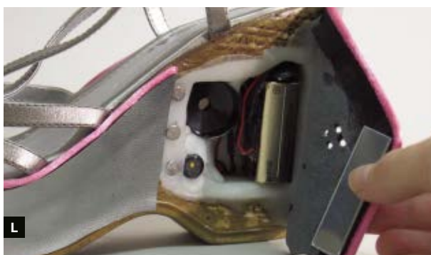
your leather. Fig. K: Mylar pattern for PMP flap includes a cutout for the PMP screen. Fig. L: Completed alarm system with holes punched in leather flap and sheet steel glued to the edge for magnetic closure.
