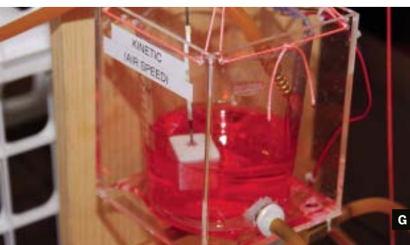
Fig. E. To fly the plane, operate the throttle and the control stick together to control the flow of energy. Fig. F: Holes in each reservoir simulate loss of energy to drag (increases with airspeed) and loss of lift from
