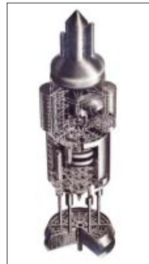
Two Mars exploration vehicles in convoy, designed by General Atomic for NASA in 1963–1964; cutaway drawing of a U.S. Air Force military payload version of a 10-meter-diameter Orion vehicle; General Atomic and the Torrey Pines mesa in La Jolla, Calif., from the air, 1964, looking north.
