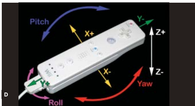
Fig. C: The OSCulator Wii-MIDI interface can associate any Wiimote actions to any MIDI commands. Fig. D: Wiimote motions: roll, pitch, and yaw.
