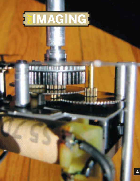
Fig. A: The clock mechanism with the aluminum spacer screwed onto the die-cut hour-hand sleeve.
