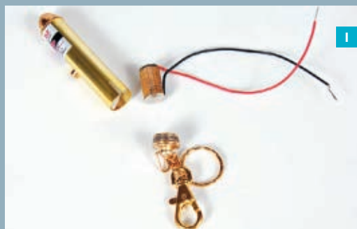
Fig. H: Measuring total current drawn by the harp lasers. Fig. I: Wooden plug power connection to the laser pointer.
