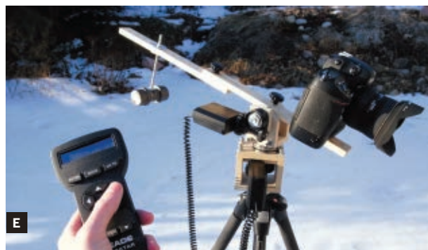
Electronic Control kit motors and worm gears installed on a homemade wooden pan/tilt head with an adjustable counterweight (you can also simply attach a camera bracket onto a Meade DS/DSM mount).
