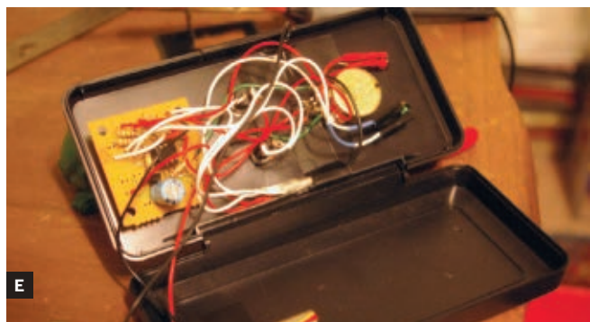
Fig. D: The underside of the board with components soldered. Fig. E: Circuit board, controls, indicators, and other components wired into a project box.
