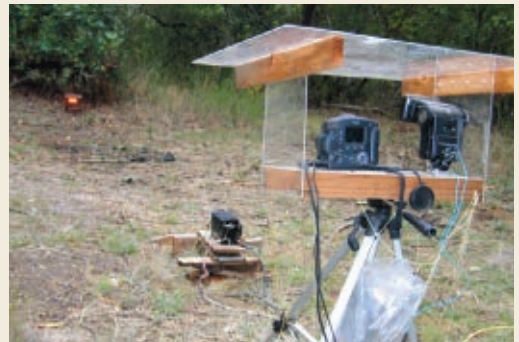
Fig. A: The camera, flash, and IR beam setup. For the circuit, go to makezine.com/15/diyimaging_wildlife .
