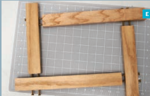
Figs. C–E: Assemble a frame to hold a bundle of conduit. For each piece, drill the 2 end holes 1\frac{1}{2} " deep with a \frac{1}{8} " drill bit, and the 4 side holes with a \frac{7}{32} " drill
