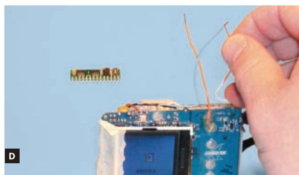
Fig. C: Soldering a wire to the on/off button-push contact (outer ring). Fig. D: Touching the shutter lead to ground (blue) takes a photo.
