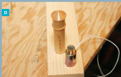
to communicate with other devices. Fig. C Install the solenoid on a wood block. Fig. D: Install pivot column.
