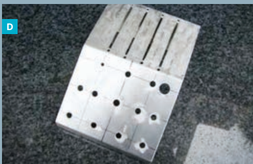
Fig. C: Toggle switches wired to button contacts on the board, and potentiometers wired to knob contacts. Fig. D: Slider, switch, and knob holes cut in the enclosure.
