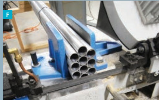
bit. Fig. F: A band saw makes swift work of cutting 10 conduits at once. Fig. G: Lengths of conduit stacked between the frames. Pieces of cable ties maintain a gap
