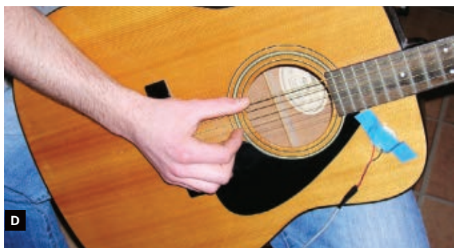
Fig. C: Could these handset earpiece speakers be repurposed as guitar pickups? Fig. D: An earpiece speaker temporarily attached to an acoustic guitar for testing.
