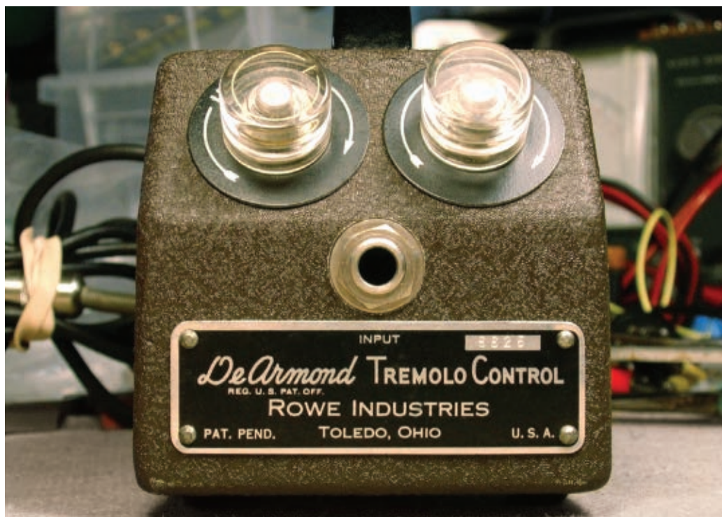
STOMP BOX 1.0: Harry DeArmond's electromechanical tremolo generator, well over 50 years old.
