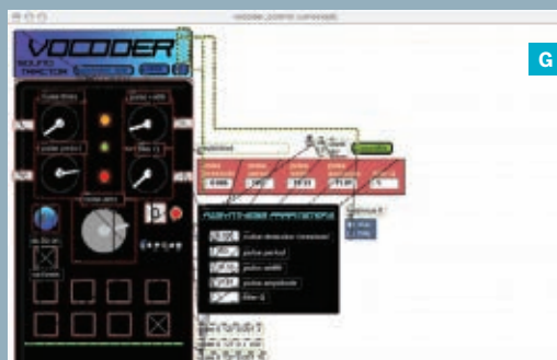
Fig. G: Inputs from the USB controller patched to a sample Vocoder app in Max.
