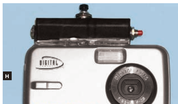
Fig. G: The paper template and cut sheet metal for the add-on control box. Fig. H: The control box glued to the top of the camera.
