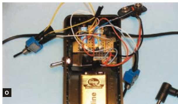
the PIC microcontroller is second from right. Fig. O: The circuit board in the enclosure with all the switches connected.
