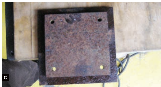
Fig. C: Drill intermediate-sized holes, working up until you get to the size hole you want. It's a perfect match!
