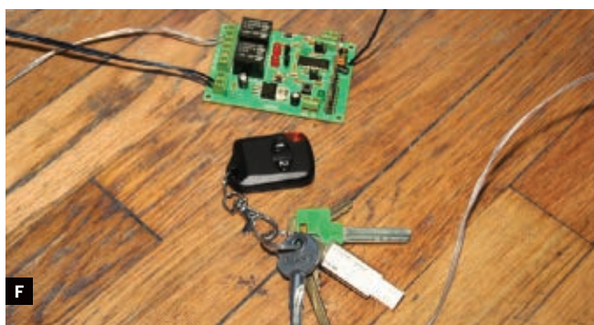
Fig. C: Panel replaced with the wire hanging down. Fig. D: Holes for power and door-signal wires drilled in the project box. Fig. E: Connected relay board in the project box. Fig. F: Relay connections and wireless key fob.
