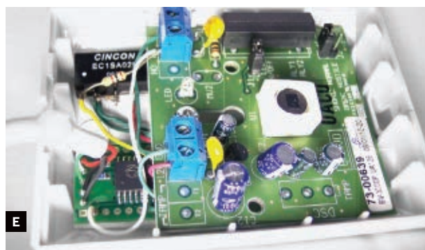
Fig. D: The wire connections to motion detector PCB terminal blocks. Fig. E: The finished circuit with the motion detector PCB back in place.
