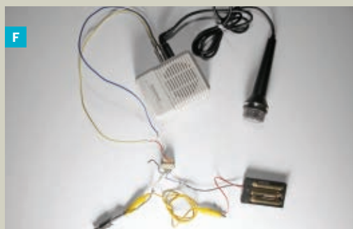
Fig. E: The photocell (i.e. photoresistor) uses battery power. Fig. F: The working transmitter is fed by a microphone.
