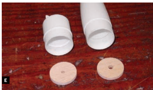
Fig. D: Mark the scale on the G-Meter dowel with contrasting colors for easy reading. Fig. E: Wooden disks for the tube coupler below the payload and the nose cone above.
