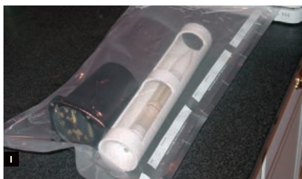
Fig. H: Calibrate the G-meter by stacking washers in multiples of carry load. Fig. I: Calibrate the altimeter alongside a working barometer or altimeter in a vacuum.
