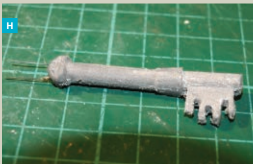
the element wire over the top of 1 half of the mold. Fig. G: The finished molding will have excess bits attached. Fig. H: Clean off the excess with a sharp knife.
