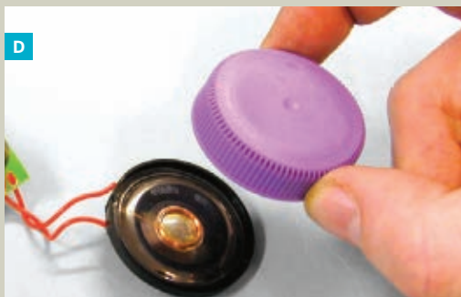
Fig C: Metal tape on the ends of the clothespin serves as contacts for the spring-loaded switch. Fig. D: A small plastic cap improves the speaker's sound.
