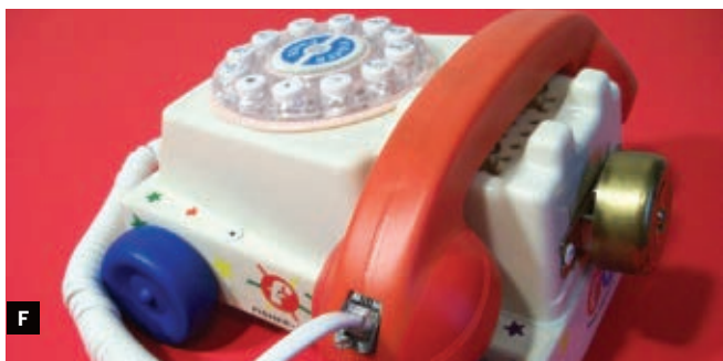
brackets for the circuit board, screw them to the board, and then pop-rivet them to the Chatter phone. Fig. F: Put the bell on the outside of the Chatter phone by pop-riveting its mount in the back.
