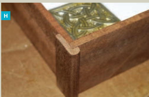
Note the small wooden stop to keep the magnet from falling out. Fig. H: Remember not to glue the corner trim to the sides!
