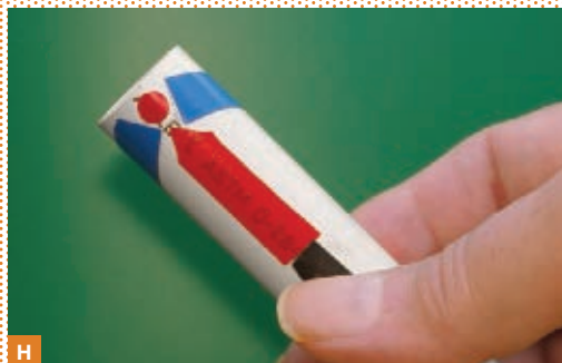
Fig. F: As the cylinder spins about its long axis, it traces a circle around the floor. When the green dot is up, the dot is moving too rapidly to be distinctly seen. The red dot moves most slowly when it is facing upward, and is therefore briefly visible, as seen from above. Fig. G: Different decorations can produce kaleidoscopic patterns. Fig. H: Experiment with patterns using colored tape.
