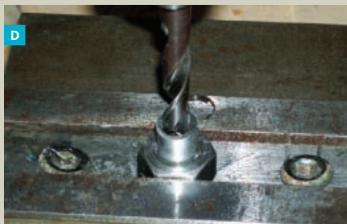
Fig. C: Use a center drill on the shank of the bolt to prevent the twist drill from “walking.” Fig. D: Hollow the shank of the bolt with a \frac{3}{8} " twist drill.
