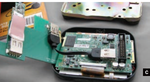
Fig. A: Chumby dissected: the original leather case, the core unit, the rear unit with Chumbilical attached, and the cotton stuffing. Fig. B: The core unit with the USB riser card in place. Fig. C: The riser circuit board
