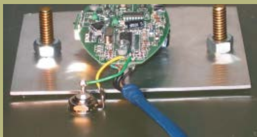
Circuit board on plate, with F connector and power line.
