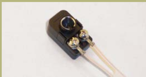
Matching transformer connected to FM antenna.
