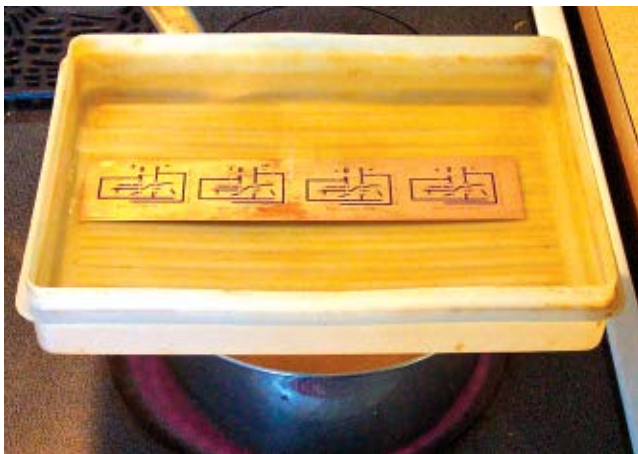
Etch the PCB on the stove.
