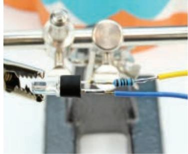
**3f.** Insulate all connections with heat-shrink tubing (I used clear heat-shrink here) or electrical tape.
