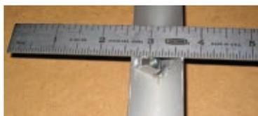
**3f.** Again at the right end of the aluminum angle, cut out a ⅜"-wide notch, 1⅝" to 1½" in from the end and on the opposite leg of the angle from the epoxied nut. On the left end of the notched leg, make a ⅜"-deep cut and bend the resulting tab outward.
