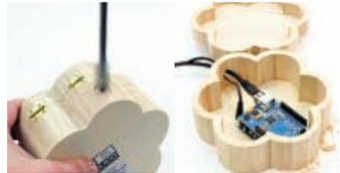
**1c.** Mark the 4 holes where you want to mount the 2 LED holders, the power switch, and the hollow wall anchor. The wall anchor should be in the center.
