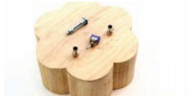
**1d.** Drill small pilot holes at each location (1/8" should work) and then drill out the holes to fit the components.
