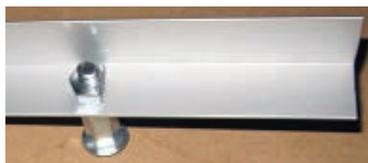
**3e.** Mix some metal epoxy and apply it generously between the nut and the inside of the boom, gluing the nut down so that its cut side faces the right end of the boom. After the epoxy cures, use a Dremel tool to grind the nut down flush with the edges of the angle, so the boom can be stored flat against the turntable.
