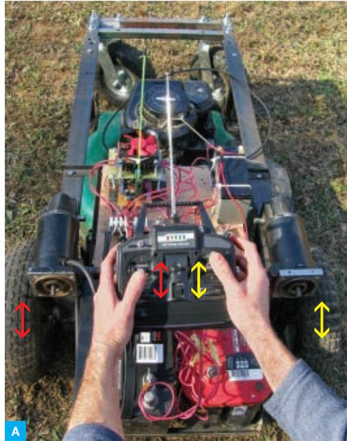
main R/C code, so you could use just one microcontroller chip with all 3 channels, but this would sacrifice some safety. If the sole ATmega goes crazy and stops responding, you're out of luck, whereas it's highly unlikely that both chips will fail at the same time. So I still use the separate, dedicated fail-safe.
