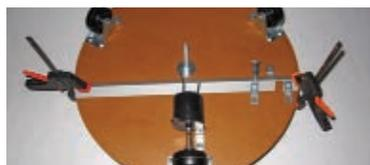
**5i.** Mark and drill #21 mounting holes for the 3 braces, countersink them on the top, and secure them with ½" flathead screws and nuts. Remove the screw with the coupling nut and adjust the braces so that the boom slides in and out easily but not freely.
