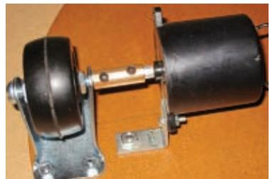
**2e.** With the turntable still inverted, lay the base disk on the wheels and check whether the motor's unused mounting flange sticks up to touch the base disk. If so, file it down to open up some clearance.
