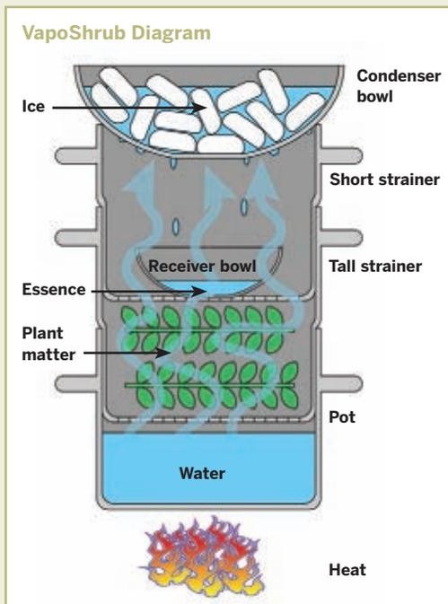
but almost any fragrant plant should work well for this project. The technique is simple: steam rises through a strainer full of plant matter, vaporizing volatile oils and other fragrant compounds, which condense on an icy bowl and drip into a small receiving bowl. Start your essence!
