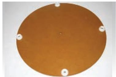
**1e.** Gently sand the top surface of the base disk and apply a third coat of polyurethane.
