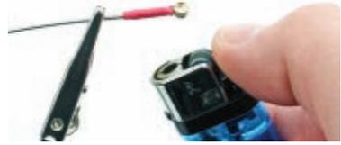
**2d.** Solder a 6" length of insulated solid-core wire (I chose red) to the brass lug grommet, extended away from the guitar string, and encase the entire connection in another piece of heat-shrink.
