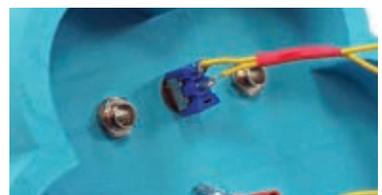
**3d.** If you're using LED holders, remove their rubber grommets and insert an LED into each. Make sure you know which color LED is which.
