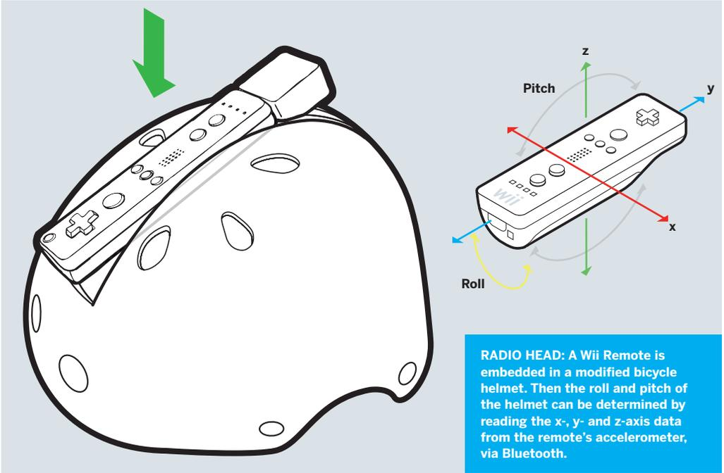
**RADIO HEAD:** A Wii Remote is embedded in a modified bicycle helmet. Then the roll and pitch of the helmet can be determined by reading the x-, y- and z-axis data from the remote's accelerometer, via Bluetooth.
