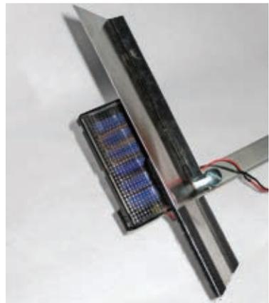
**4f.** Test-assemble the boom, cell, and shade. Velcro the PV cell to the end of the boom, then fasten the coupling screw and nut to the boom through the mounting hole in the shade. The shade should sit tilted over the PV cell, and the cell's wires should thread through the slot in the boom.
