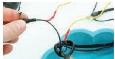
**3c.** Solder the free ends of the wires you just attached to the 2 terminals of your switch. No need to worry about the polarity; either way works.
