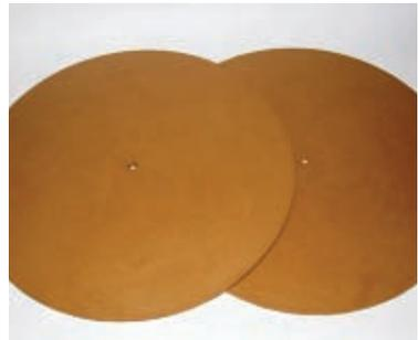
**1c.** Brush a polyurethane sealer over each disk, let dry, and add a second coat. Repeat on the other sides and around the edges.
