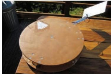
**6b.** Place the platform on a flat surface in the sun and orient it so that the entire PV cell is illuminated. If the wiring is correct, the turntable should rotate clockwise until the surface of the PV cell is only partially illuminated. Tracking has begun! But if the turntable rotates counterclockwise (and you're in the Northern Hemisphere), you need to swap the motor connections. Solder them when they're correct, and cover them with electrical tape.
