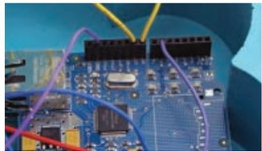
**4b.** To wire the split lead from the wall anchor, plug the lead without the resistor into Arduino digital pin 6, and the resistor lead into ground. All done!
