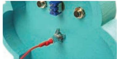
**2f.** While keeping the guitar string centered (I used a "third hand" but you could have a friend hold it steady), apply some hot glue into the core of the hollow wall anchor around the string. You don't want to fill the entire cavity, just a bit around the bottom to further insulate the guitar string and keep it straight and secure. If you add too much hot glue, the wire won't be able to flex enough to touch the top of the anchor, so err on the side of caution and use only a dab or two.
