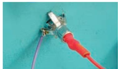
**2i.** Now we'll split the connection from the hollow wall anchor so that one wire goes to an Arduino ground pin (GND) through a 10kΩ resistor, and the other wire connects to its digital I/O pin 6. Doing this pulls pin 6 to ground, so that it reads LOW unless contact is made by the sensor.
