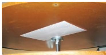
**5c.** With the turntable still inverted, install the ¼-20 stop nut, and make sure the disks can rotate freely. Measure how much of the 3½" axle protrudes above the stop nut. Disassemble the turntable, cut off this protrusion, and file the end smooth.
