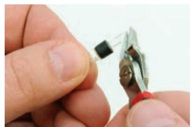
**3e.** For each LED, solder a  $220\Omega$  resistor (or similar value) between the positive (longer) lead and a 3"–4" length of wire. The resistor limits the amount of current that flows through the LED, so that it won't burn out. Solder a 3"–4" wire of a different color to each negative lead. I used yellow for positive and blue for negative, but red and black are traditional.
