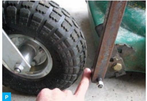
side. The drive wheels have built-in bearings, so they attach onto the ends of the axle with another nut, sprocket side in.
