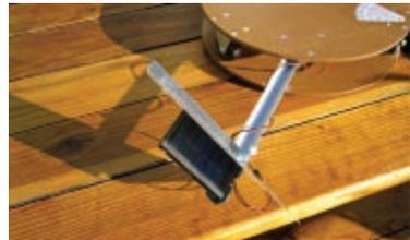
**6c.** To determine the platform's central tracking angle — its optimum orientation — install the brass tube (the gnomon) in its hole and position the tracker so that its PV cell is fully lit by the sun. Watch it for several cycles, noting the shadow's positions on the protractor when the motor starts and stops. The average between these 2 readings is the central tracking angle.
