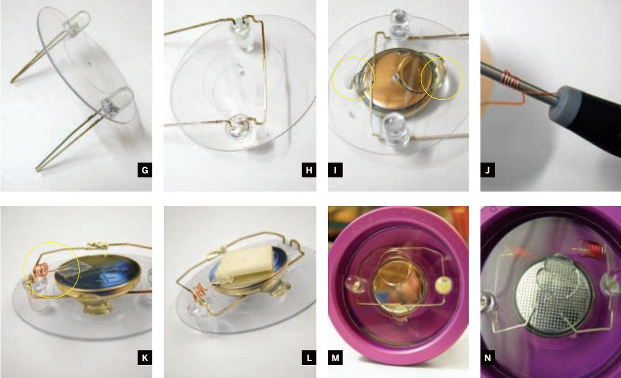
Fig. G: LEDs press-fit into holes. Fig. H: Bend the LEDs' negative leads to meet. Fig. I: Glue the battery's negative side to the cap so the negative leads are touching it. Fig. J: Coil wire around a small screwdriver to make a
