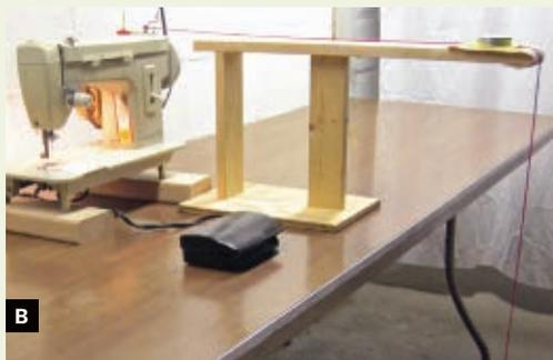
lower than the bottom of the bobbin winder, and hanging over the front edge of your work surface (Figure B). Round off the front edge of the platform and cover it with felt. The spool of magnet wire sits underneath this edge on the floor.
