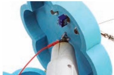
**2g.** Feed the Ethernet and power cables through the hole you drilled in Step 1b. Tie a simple knot to keep them from being pulled out of the box. Position the Arduino boards in the box, plug in both cables, and also plug the red wire from the guitar string into its 5V header socket.
