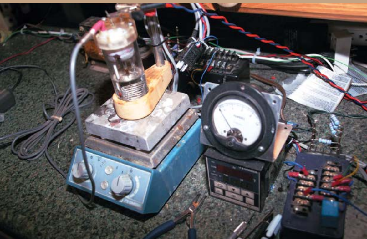
Above: A Seebeck calorimeter opened to expose an electrolytic cell in which heat may be generated by low-energy nuclear reactions. Below: Inside this cell, metals can be plated onto the surface of palladium wafers.
