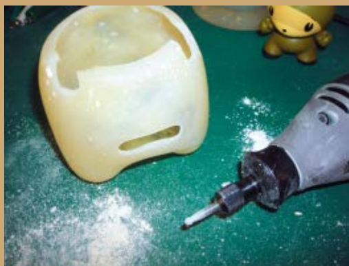
After the resin cures, you can use a Dremel tool to machine the base.
