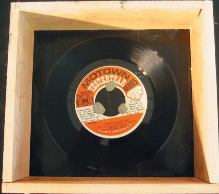
Fig. 1: Place the record you want to duplicate in a box that has been taped up along the corner edges to prevent leakage. You'll then pour enough liquid silicone into
