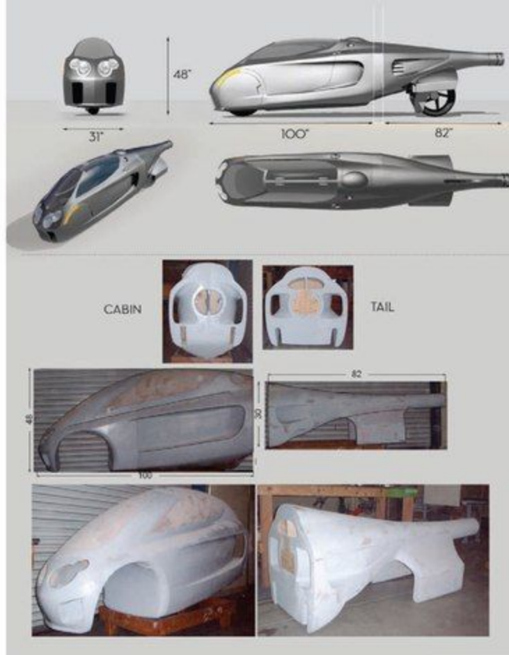
(Right) Plugs for casting composite body panels for the GT. (Below) The geometry of a street-legal gyrocycle guides the progression of the GT's fairing design.
