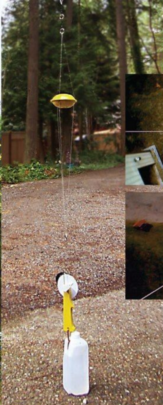
(Far left) Easy-to-start camera timer. (Left) Reel clips to the water-filled bottle, and anchors the balloons as the saucer hangs chest-high off the ground, making it easy to check the batteries inside. (Right) Balloon Cam Success!
