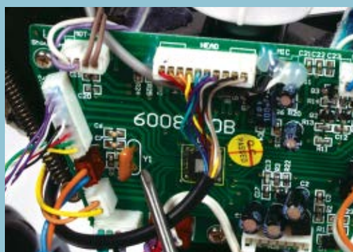
The Robosapien main circuit board is located on the robot's back. The crystal capacitor is labeled Y1.
