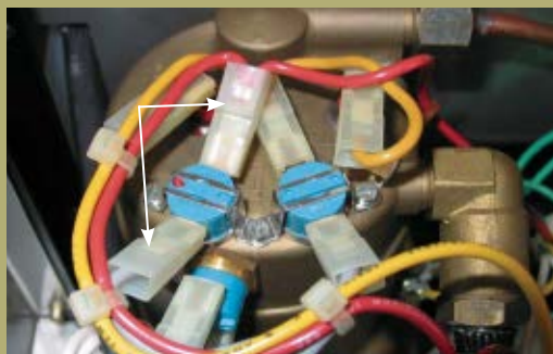
Fig. 2 Removing brew thermostat connectors.
