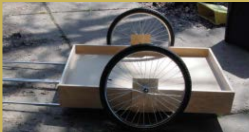
The cart uses standard 26" bicycle wheels.
