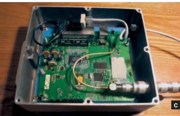
Fig. A: Popping the Linksys router apart. Fig. B: Our antenna connector, cut off from the router's circuit board. Fig. C: Inside the case, at upper left, are electrical tape-wrapped Power over Ethernet (PoE) adapter hooks
