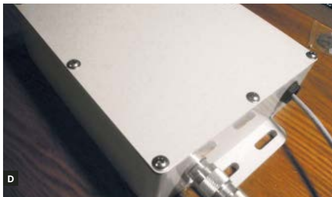
up to router RJ-45 and power ports; at lower right, the board's antenna connector plugs into an N adapter and bulkhead connector which take the connect outside. Fig. D: The sealed case.
