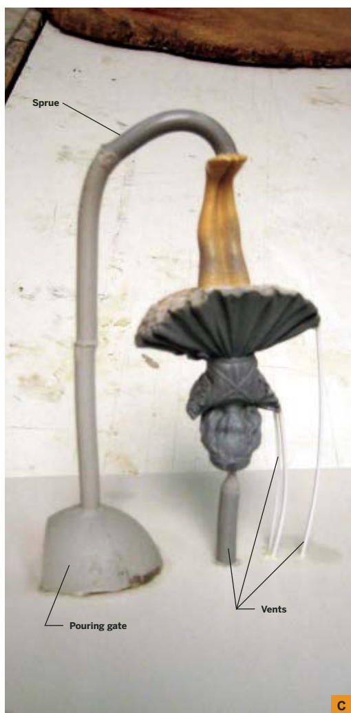
Fig. A: Cross section of underpoured mold. Fig. B: The object we're going to cast, an angel figurine. Fig. C: The angel being set up for molding. The sprue runs to her feet, which are a conveniently flat surface. Fig. D: Marking the parting line, along which the mold will be cut later. Fig. E: Building the mold box using a single piece of foamcore. Fig. F: The mold box, ready for sealing with hot glue.
