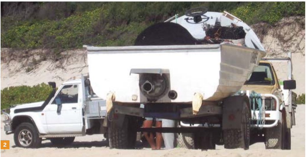
1. Charlie Asquith and his dory. 2. The jet nozzle and exhaust at the stern of the boat. The boat goes faster than the jet ski did and gets better gas mileage. This jet ski engine is about 100 horsepower. The white truck (left in photo) has a snorkel so the engine can still run while the truck is nearly underwater. 3. The skipper stands in the front with the controls from the jet ski.
