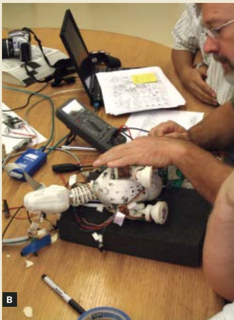
A. The Anatomy of the Furby by artist Kelly Heaton, who once made an interactive Furby wall. B. A Ugobe engineer troubleshoots a locomotion problem with Pleo. C. Caleb Chung's lab is an unassuming box in a small office park outside of Boise. D. A Pleo tail-testing unit. E. Pleo in a classic pose.
