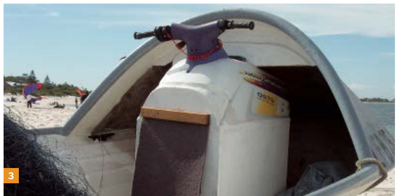
1. Charlie Asquith and his dory. 2. The jet nozzle and exhaust at the stern of the boat. The boat goes faster than the jet ski did and gets better gas mileage. This jet ski engine is about 100 horsepower. The white truck (left in photo) has a snorkel so the engine can still run while the truck is nearly underwater. 3. The skipper stands in the front with the controls from the jet ski.
