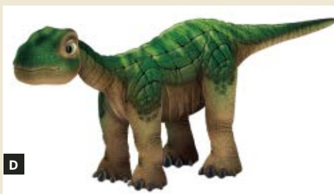
A. Pleo is a proportionately correct baby camarasaurus robot. B. An exoskeleton provides support. C. Motors, gears, and linkages provide realistic movement. D. Sight, sound, and touch sensors are hidden under the hide.
