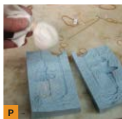
Fig. J: The mold, ready to be cut out. Fig. K: Cutting the box seam. Fig. L: The mold, released. Fig. M: The jeweler's cut. Fig. N: Prying the halves apart. Fig. O: The angel revealed (with vents, etc. removed). Fig. P: Dusting the mold with release agent (cornstarch or talcum powder).
