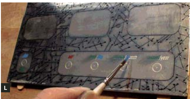
Fig. K: Filling in the etched arrow details with a fine paintbrush and black enamel paint. Fig. L: Filling in the color detail with more enamel.
