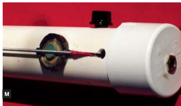
Fig. L: Install the wedged rubber-stopper nut.
