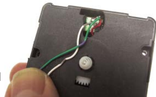
Fig. C: New wires to your own circuit connect to the electromagnet through the clearance hole in the now-bare clock face.
