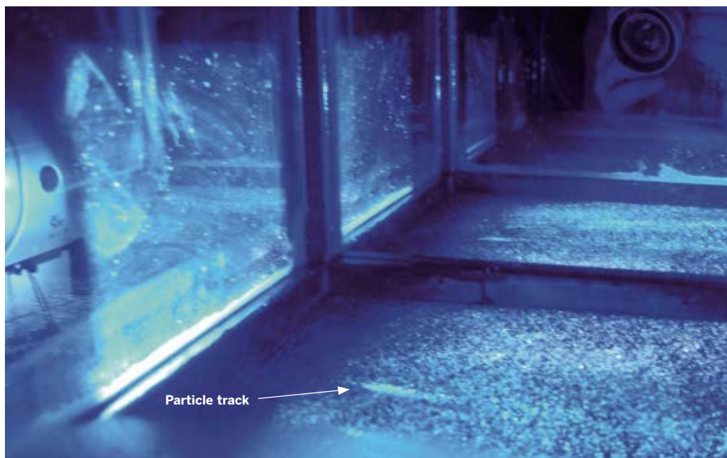
Inside the trophy case cloud chamber when chilled and illuminated by an LCD projector. Although they do not show up well in this photograph, the alcohol droplets and particle tracks are clearly visible to the naked eye.
