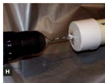
(3) Lag screws are used as strap buttons. Fig. F: Prepare the pickup by cutting away the top of the plastic case. Fig. G: Attach a rubber foot in the disk center. Fig. H: Drill the cap. Fig. I: Sand one side flat.
