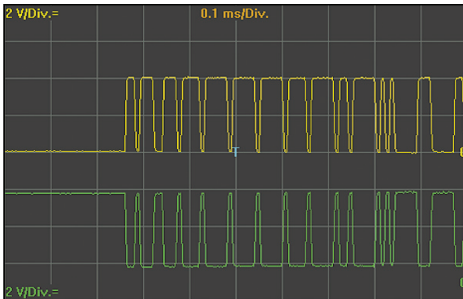
Signal Pattern Image on VAS 5051 DSO (Freeze Frame)
