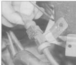
6.2 Removing the turbo over-pressure warning switch
