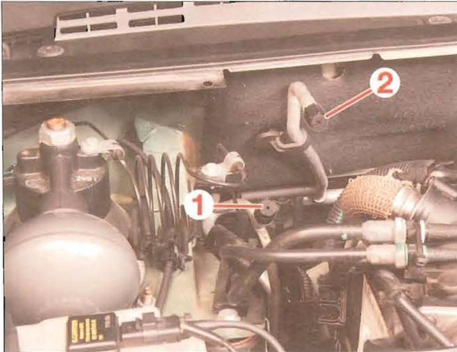
**SITUATION DES RACCORDS DE SERVICE HAUTE (1) ET BASSE (2) PRESSION DU CIRCUIT DE CLIMATISATION**
