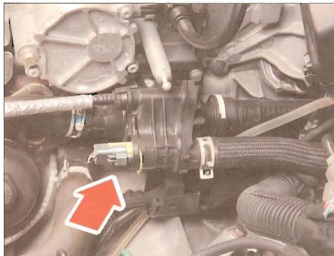
**SITUATION DE LA SONDE DE TEMPÉRATURE SUR LE BOÎTIER THERMOSTATIQUE**
