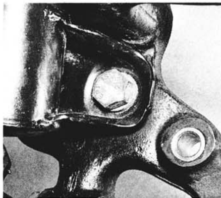
5.7a Strut-to-steering knuckle lower front bolt
