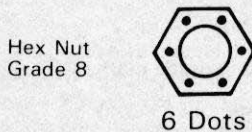
Standard hex nut strength markings
