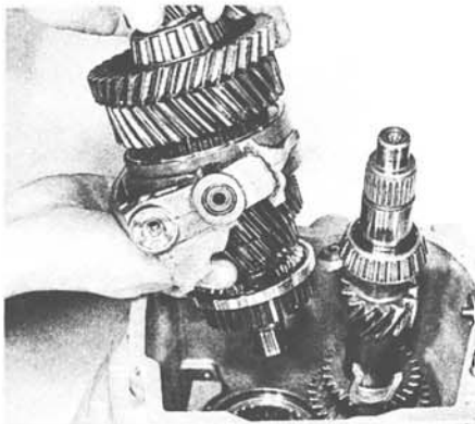
12.12a Locate the mainshaft assembly in position ...
