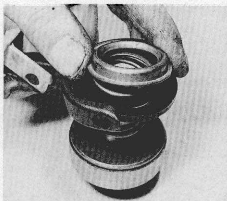
11.16b Lift off the retaining cap
