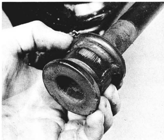
12.4 The anti-roll bar bushing can be slid off the bar – if its old and hardened, cut it off
