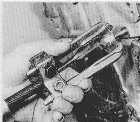
10.27b Use a puller and slide hammer arrangement to remove the slide rail bearing bolts
