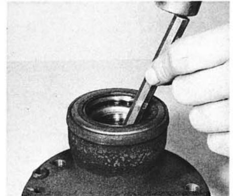
4.12 If the bearings are to be replaced, knock the outer races from the hub using a long drift
