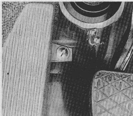
40.9 Pry off the footrest retaining spire clip – if this is done carefully, the clip can be reused
