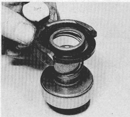
11.16c Remove the actuating lever
