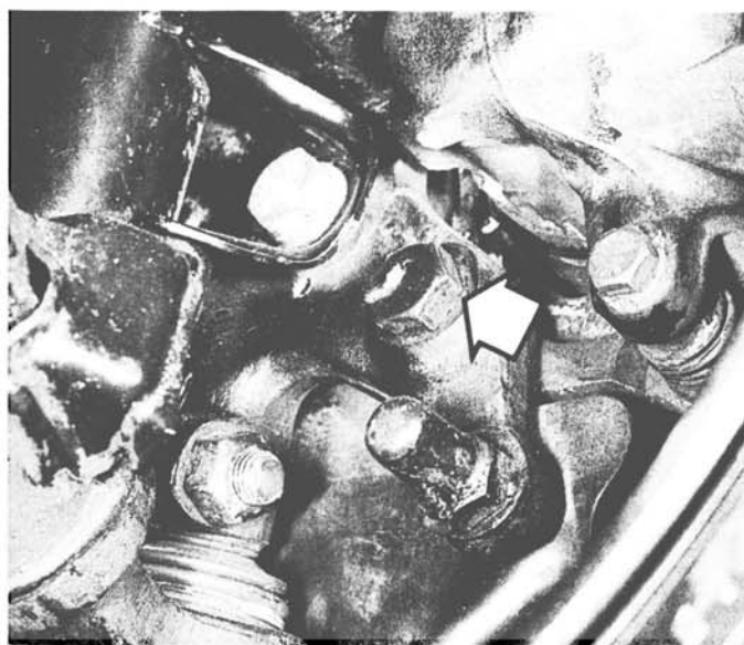
4.6 Lower mounting bolt of the caliper carrier (arrow)
