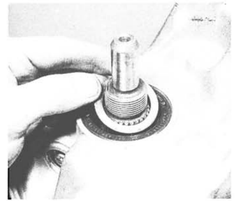
12.29a Install the spacing washer over the end of the output shaft
