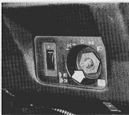
42.8 Remove the light switch retaining nut (arrow)
