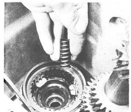
12.6a If equipped, place the preload spring in the input shaft bore . . .
