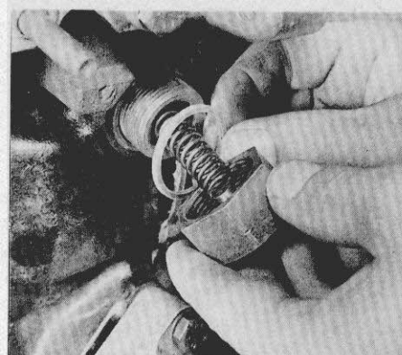
8.8B Remove the tensioner spring and sealing ring
