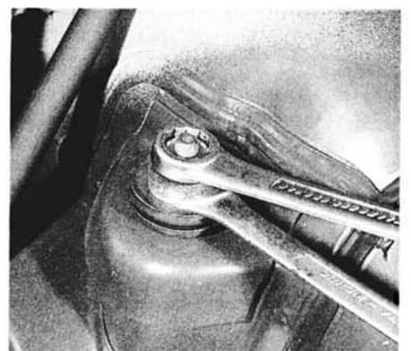
21.7 Loosen the shock absorber mounting locknuts
