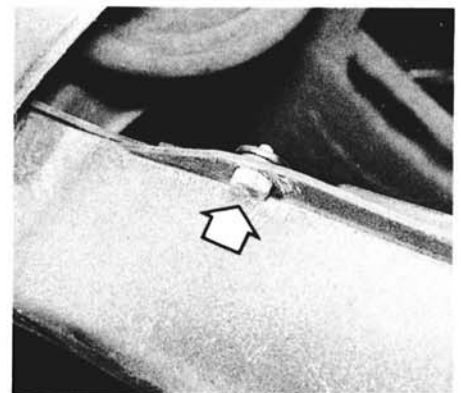
21.2 Spring support arm cover retaining bolt (arrow)
