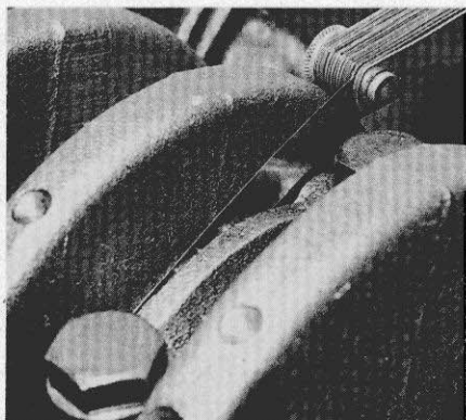
25.14 Checking crankshaft endplay with a feeler gauge
