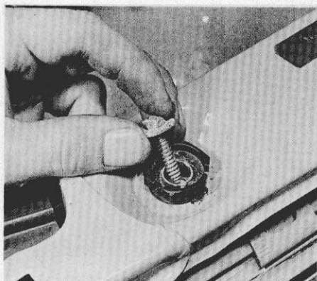
23.8a Remove the upper retaining bolts . . .
