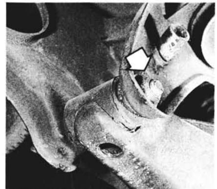
19.4a Loosen the spring support arm inner mounting nut (arrow)
