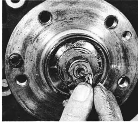
4.7 Remove the radio interference contact spring
