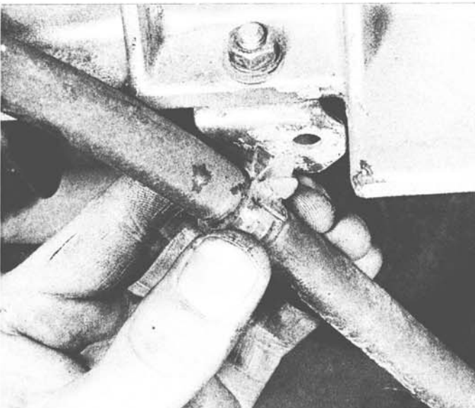
3.16 Detach the speedometer cable clips from the brackets
