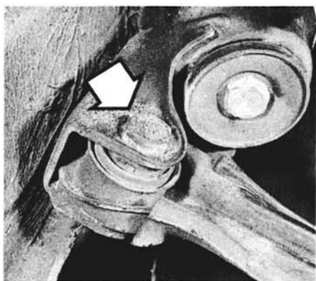
17.3 Pushing strut-to-subframe retaining bolt (arrow)
