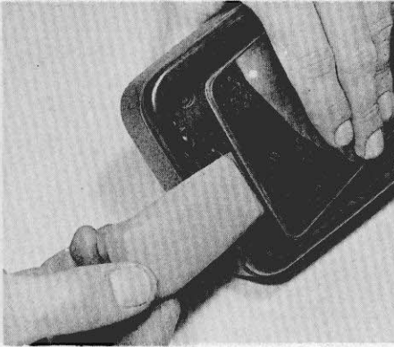
31.1a Pry out the mirror glass using a plastic wedge . . .
