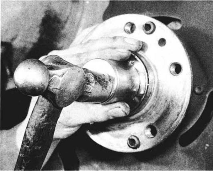
4.19 Tap the hub onto the spindle using a large socket or piece of pipe
