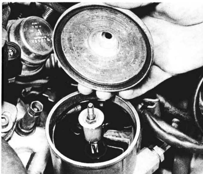
2.10 The fluid level should be up to the punched or cast mark on the reservoir
