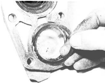
12.1 Install the spacer washers in the front cover
