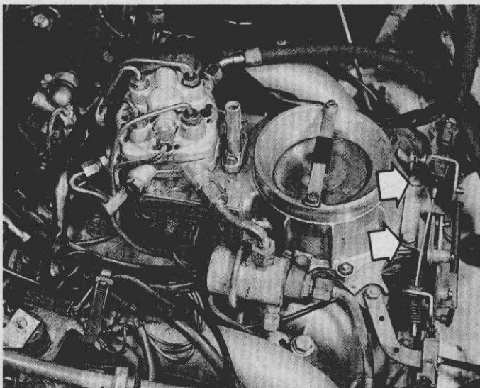
18.2 Throttle linkage bracket retaining bolts (arrows)
