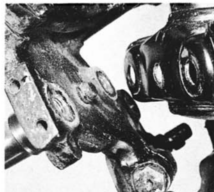
6.4b Removing the suspension strut from the steering knuckle
