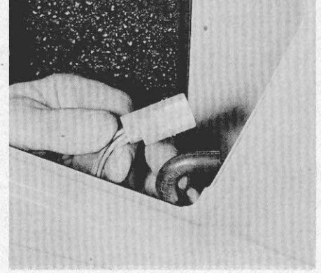
25.3c Disconnect the wiring and vacuum hose at the solenoid
