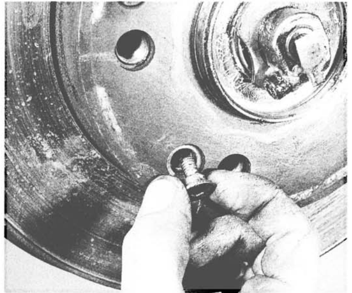
6.7 The front brake disc is held to the hub with an Allen-head screw
