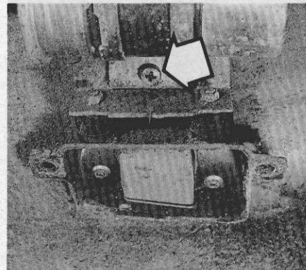
10.9 Filter retaining strap screw
