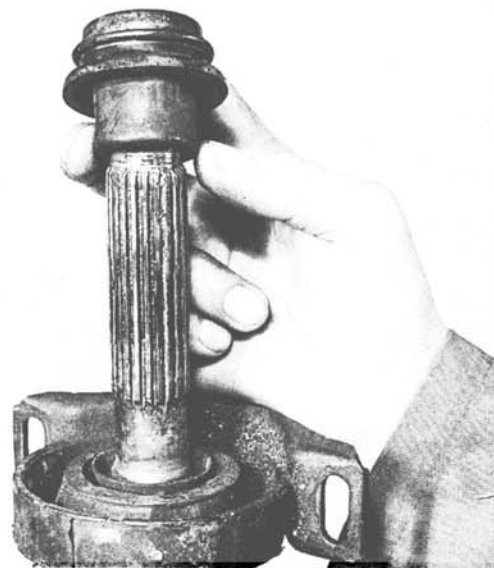
5.3 Slide the rubber boot off the driveshaft splines
