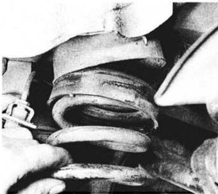
19.12a Install the spring in its upper mount . . .
