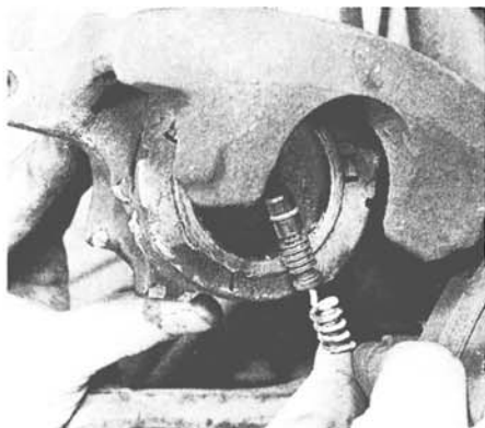
3.5b Pivot the caliper up for access to the brake pads
