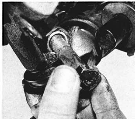
5.9 Remove the steering knuckle-to-control arm nut and pinch-bolt
