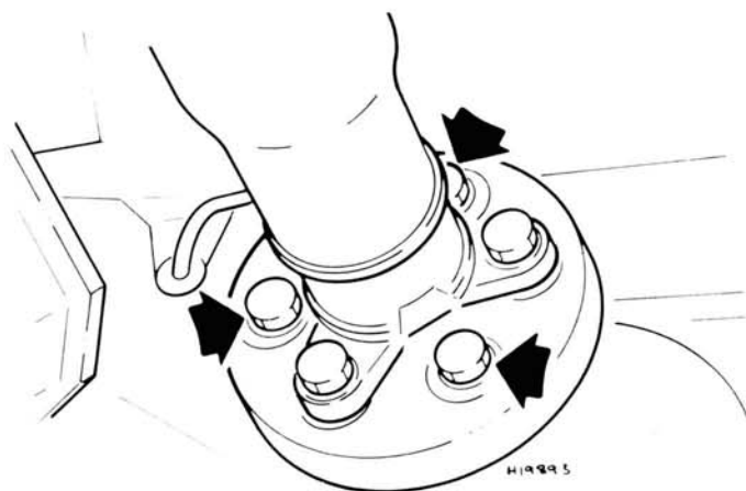
3.6 Driveshaft rear flexible coupling-to-differential flange retaining bolts (arrows)
