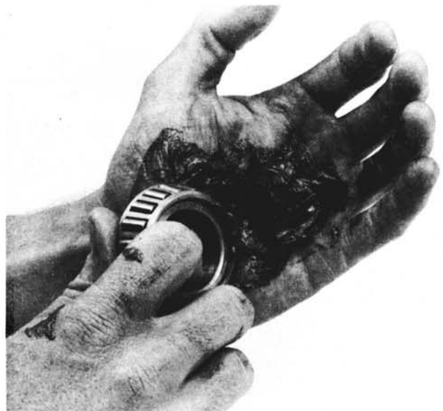
4.16 Work the grease completely into the rollers
