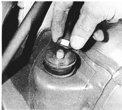
21.8 Remove the nuts, washer, bushing and bushing seat
