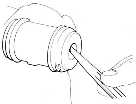
9.4 Use a punch to knock out the control arm front bushing sleeve
