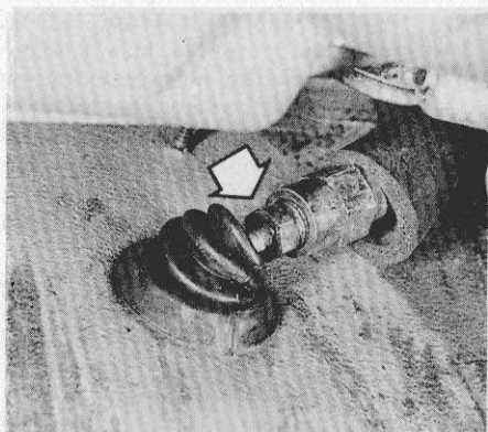
4.2 Unscrew the slave cylinder rigid line-to-flexible hose fitting
