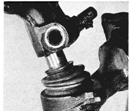
5.10 Withdraw the steering knuckle from the control arm balljoint – if it's stuck, spread the pinch joint gap with a screwdriver
