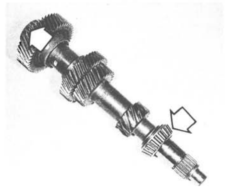
8.1 Tapered roller bearing locations (arrows) on the layshaft
