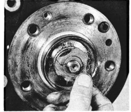
4.8 Remove the hub nut and thrust washer
