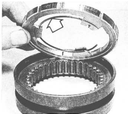
11.4 Check the condition of the synchro ring and annular spring (arrow)
