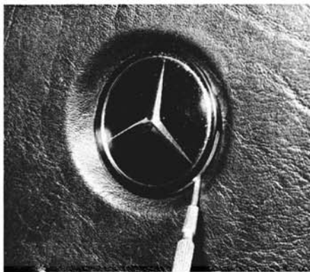
23.2 Pry out the steering wheel trim motif
