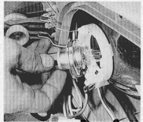
21.3 Remove the bulb from the headlight
