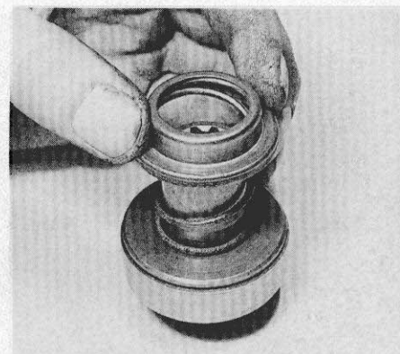
11.16d Lift off the inner cap
