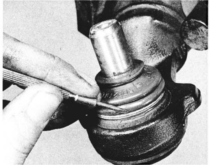
10.2 Use a small screwdriver to pry out the balljoint dust boot retaining clip
