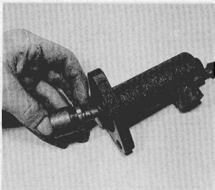
5.3a Pull out the slave cylinder piston . . .
