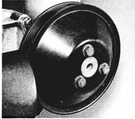
29.8 Power steering pulley-to-pump flange retaining bolts
