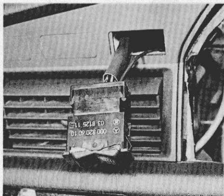
16.3 Pry out the switch and disconnect the electrical connector
