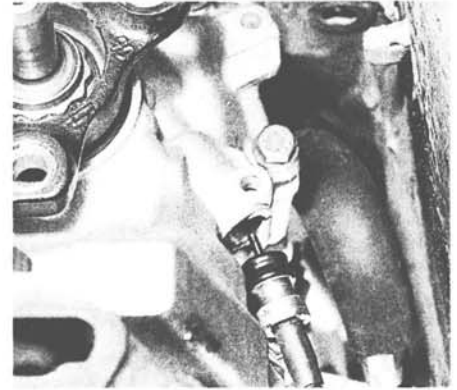
3.15 Removing the speedometer cable
