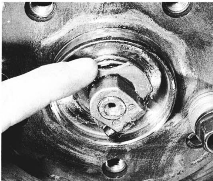
3.8 The hub bearing adjustment is correct if the thrust washer can just be moved with one finger
