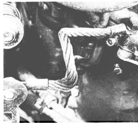
23.32 Engine ground strap attachment at the transmission
