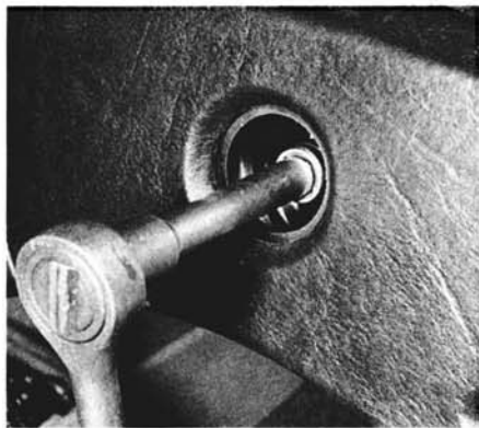
23.3 Remove the retaining bolt with an Allen wrench socket
