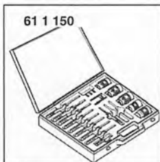
➤ Wiring harness repair kit (BMW special tool 61 1 150)
