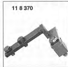
Engine block support tool (BMW special tool 11 8 370)
