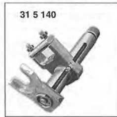
Control arm removal and installation tool (BMW special tool 31 5 140)
