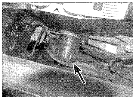
3.6 On 1.4 litre engines, the oil filter is located on the front of the engine
