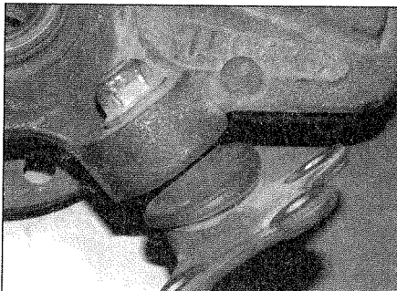
6.2a The front suspension lower balljoint on the wheel bearing housing
