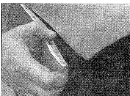
6.6 Ease the rear ends of the bumper from the guides
