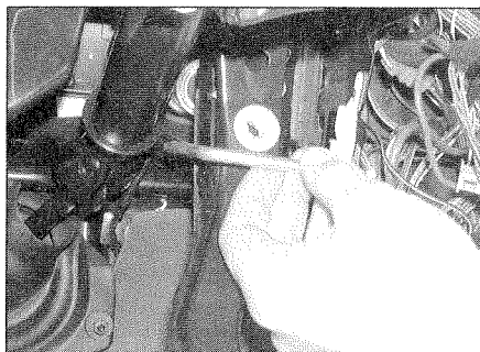
13.5b Using the tool to release the brake pedal from the servo pushrod
