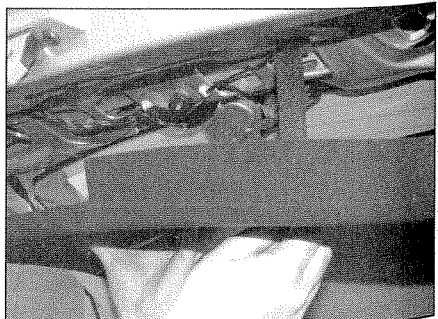
16.2 Removing the tailgate trim panel
