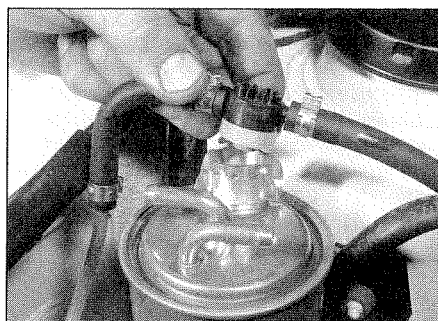
10.2b . . . and lift out the control valve, leaving the fuel hoses attached to it
