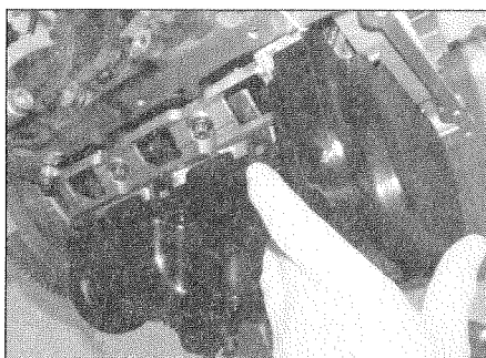
21.6a Remove the plastic cover/strainer from the bottom of the crankcase . . .
