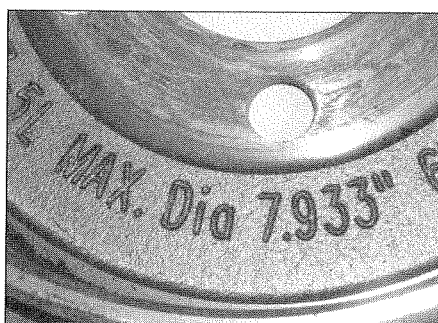
10.6 The maximum diameter of the drum is stamped on its inner surface
