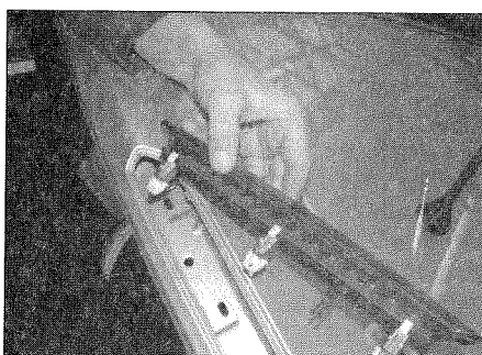
5.59b ... and remove the high-level brake light
