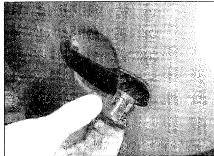
13.10 Pull out the housing and cap ...
