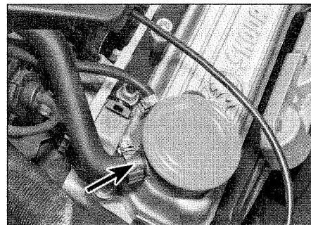
4.7 Replace the original Skoda clips with screw-type clips when refitting
