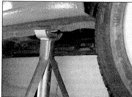
Use an axle stand with a suitable block of wood
