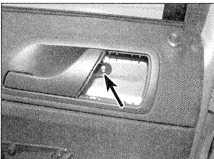
12.15b ... then unscrew the upper bolt securing the inner trim panel
