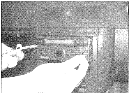
21.3a Insert the keys and pull out the radio/cassette player
