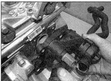
4.5 Removing the coolant distribution housing from the cylinder block
