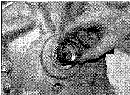
12.5a Locate the new oil seal in the timing cover . . .
