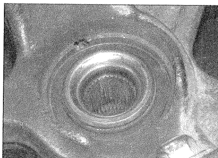
3.7b Make sure the circlip is fully entered in its groove
