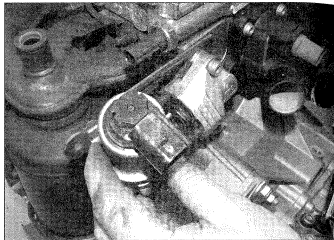
4.5c ... and remove the EGR valve from the adapter – engine code BME
