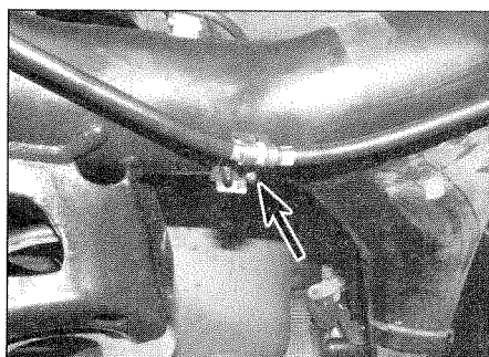
19.4a Handbrake cable fixing on the rear trailing arm
