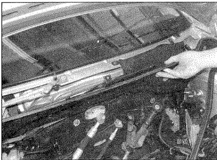
18.3b ... and remove the engine compartment rear panel from the bulkhead
