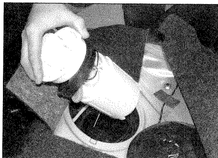
6.9a Lift out the pump/sender unit . . .
