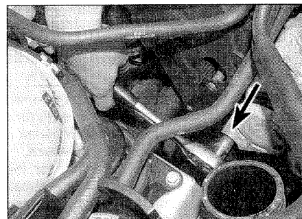
29.4 On models with air conditioning, turn the tensioner clockwise ...
