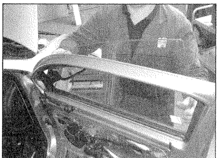
15.7 Removing the front door window glass
