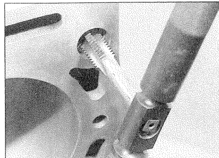
12.7 To clean the cylinder block threads, run a correct-size tap into the holes
