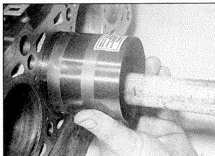
19.13 Using a hammer handle to tap the piston into its bore
