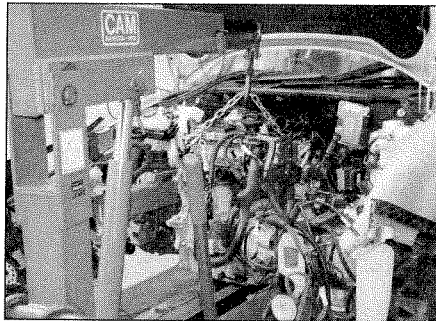
4.25 Removing the engine/transmission assembly – diesel engine code AMF
