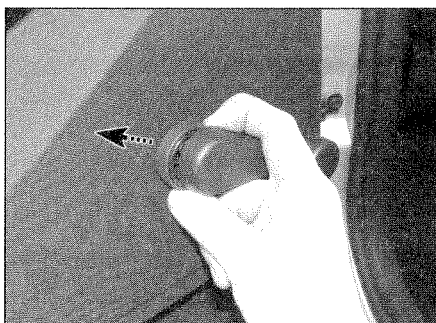
12.11 Remove the window crank ...
