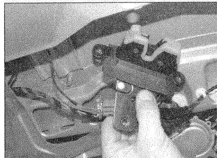
17.2b . . . withdraw the tailgate lock . . .
