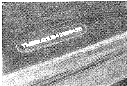
Vehicle Identification Number (VIN) located on the left-hand front edge of the windscreen
