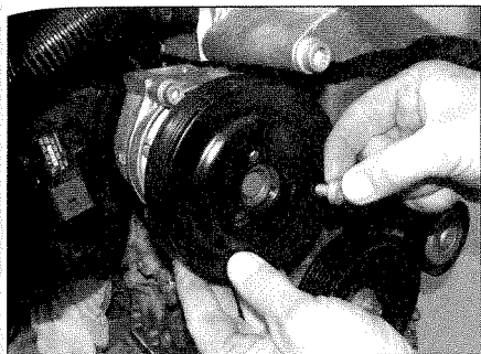
7.4 Removing the coolant pump pulley – engine code BME
