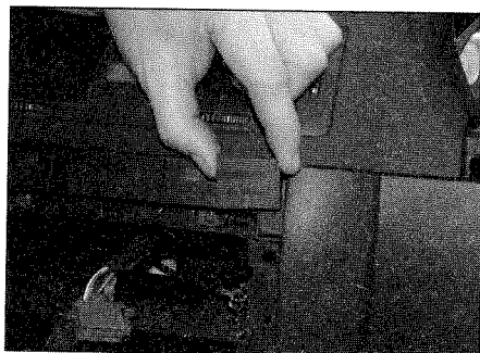
29.13 Removing a switch blank from the fascia
