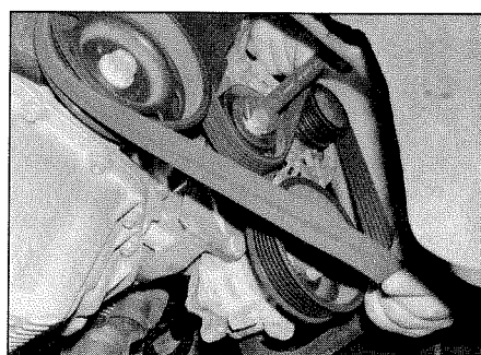
26.6 Auxiliary drivebelt removal – 1.4 litre DOHC engine with air conditioning
