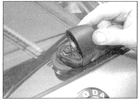
17.5a Pull up the spindle nut cover ...
