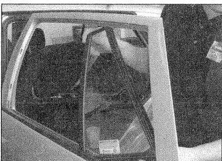
15.9b . . . and withdraw the quarter light from the rear door
