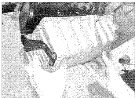
14.6 Removing the sump – engine code AMF
