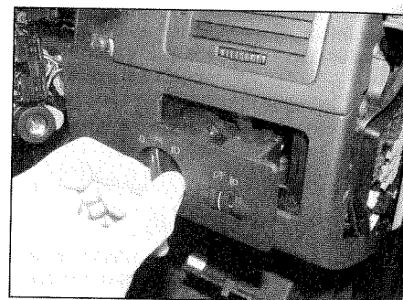
4.8b ... then pull the switch from the dash ...
