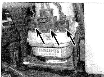
22.8 Wiring plugs on the electric power steering pump
