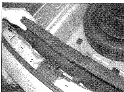
17.3b Removing the trim panel from the rear valance . . .
