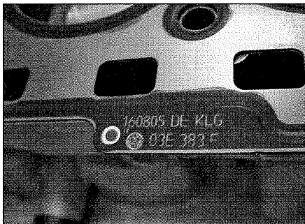
8.17c Typical cylinder head gasket markings
