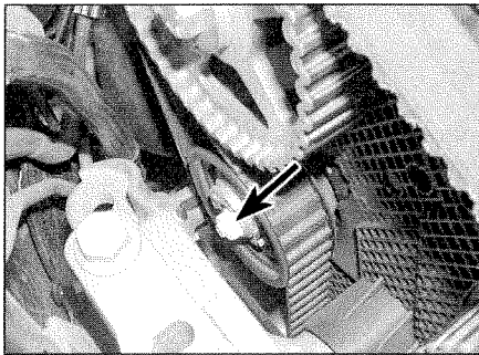
8.2 Timing belt tensioner nut – engine code ASY
