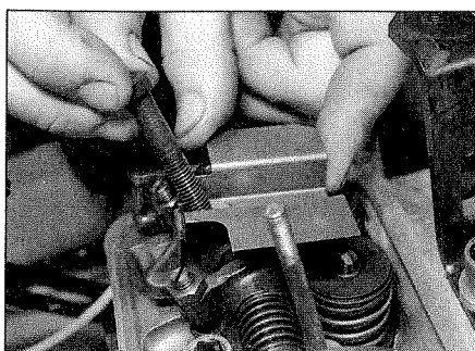
5.10a Don't forget to refit the oil splash plate to the right-hand pedestal
