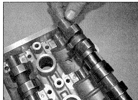
7.28 Removing the camshafts from the cylinder head cover
