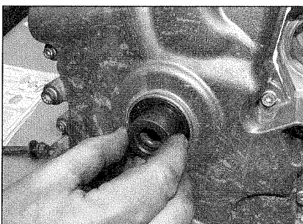
12.6b . . . and insert the sleeve
