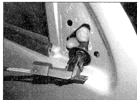
20.5c . . . while guiding the control cables through the door
