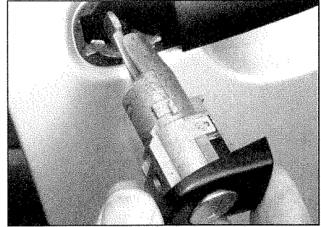
13.5 ... pull out the lock cylinder and cap ...
