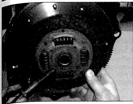
6.11 Locating the friction disc on the flywheel
