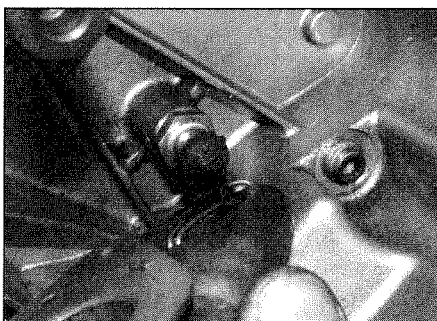
7.12 Locating the release lever and spring onto the ball-stud
