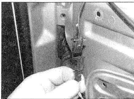
20.4a Disconnect the mirror wiring connector . . .
