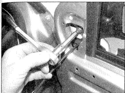
20.5a Undo the mounting screw . . .
