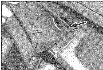
12.3a Use a small screwdriver to release the plastic clip on the oddments holder (manual window shown)
