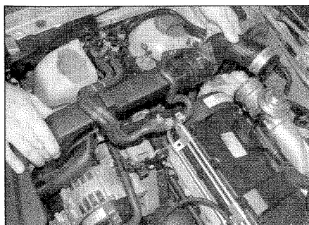
6.1 Removing the air intake hose from across the top of the timing belt cover
