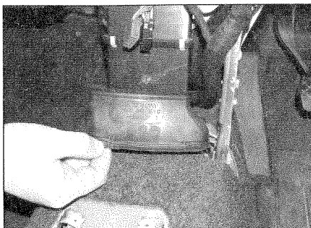
9.16b ... and bottom air vent from the heater assembly
