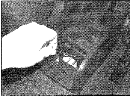
17.3 On some models, access to the handbrake adjusting nut can be gained by removing the ashtray
