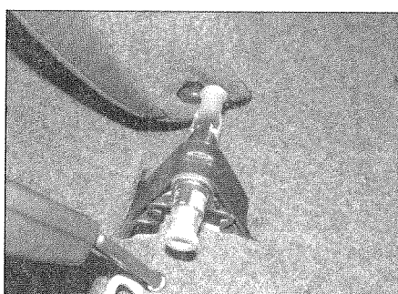
24.12 Slide the backrest from the pivot pin
