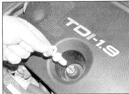
4.9c ... on this engine, the dipstick has to be removed ...
