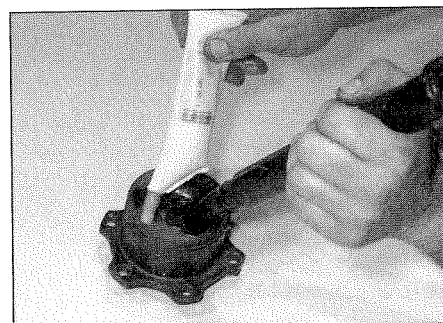
3.34 Work the grease into the joint outer member
