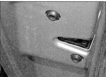
14.2 Screws securing the door lock to the rear edge of the door
