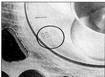
13.25a The piston crown is marked with an arrow which must point towards the timing belt end of the engine
