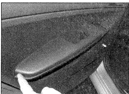
12.13 ... slide the rear cover forwards ...
