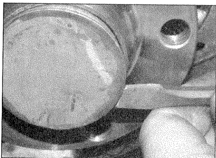
9.3 Use a cold chisel or screwdriver to remove the rear hub dust cap
