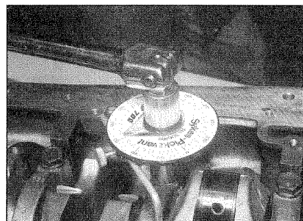
18.12b ... then through the specified angle
