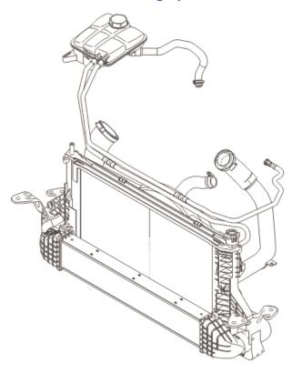
The coolant pump pumps coolant through the cylinder block, and also cools the cylinder head, cylinder sleeves, spark plug wells, intake ducts and fuel injection nozzles.
