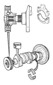
The crankshaft has six main bearings. The 5th main bearing is a throw-out bearing. At the front end of the crankshaft are two spline joints, the inner of which drives the oil pump. The drive gear for the timing belt and vibration damper is on the outer joint.
