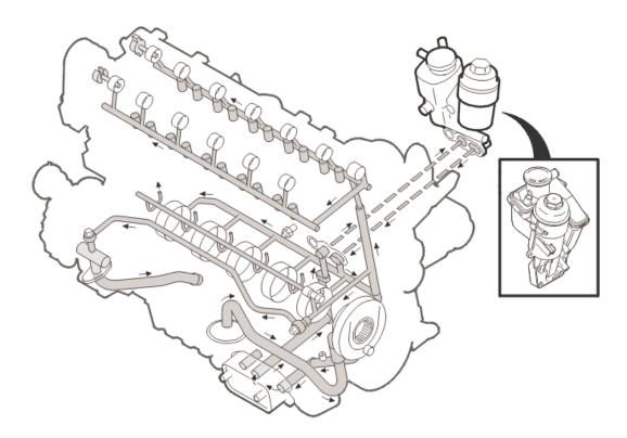
The oil is led from the oil pan via a suction nozzle to the oil pump. The oil pump is located on the engine block. The oil is then pumped onwards to the oil cooling system and then to the oil filter.
