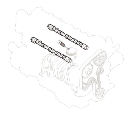
The camshafts are cast iron. The cams lobes which press against the valve lifters are harder to tolerate the contact pressure. The valve lifters are steel and mechanical, not hydraulic.
