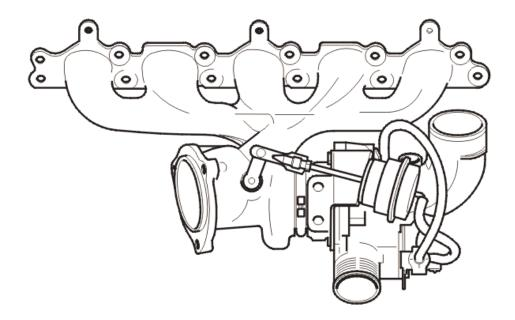
The integrated manifold and turbine housing are made of austenite forged steel to tolerate exhaust temperatures up to 1050 °C.
