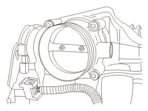
The throttle body (TB) is die cast aluminum. The throttle disc is brass on naturally aspirated engines and aluminum on turbocharged engines. The position sensors are under the plastic cover. These read the position of the throttle disc. There are also two connections to the engine in the cover. These turn the throttle disc to the angle requested by the driver.
