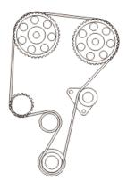
The tensioner consists or a spring and a friction element. The friction element provides the required damping to absorb small oscillations and speed variations. The spring ensures correct belt tension, irrespective of wear and temperature. The belts are made of cord reinforced rubber.
