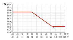
To charge the battery optimally the central electronic module (CEM) calculates the output voltage from the generator (GEN) using the temperature of the battery. The alternator control module (ACM) controls the output voltage, depending on the control from the central electronic module (CEM). See the illustration above. In some driving conditions for example, the engine control module (ECM) is able to affect generator (GEN) control, whereby the output voltage will deviate from the above.
