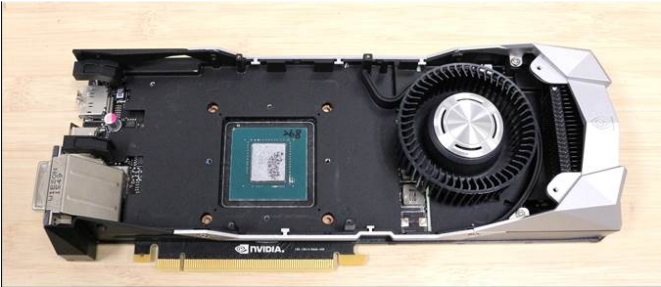
Figure 2n: Align the baseplate on topside of the board with orientation as shown. Note: Do NOT hold/hit the fan at anytime during assembly. Recommend to use a supporting fixture. Handle with care is required.
