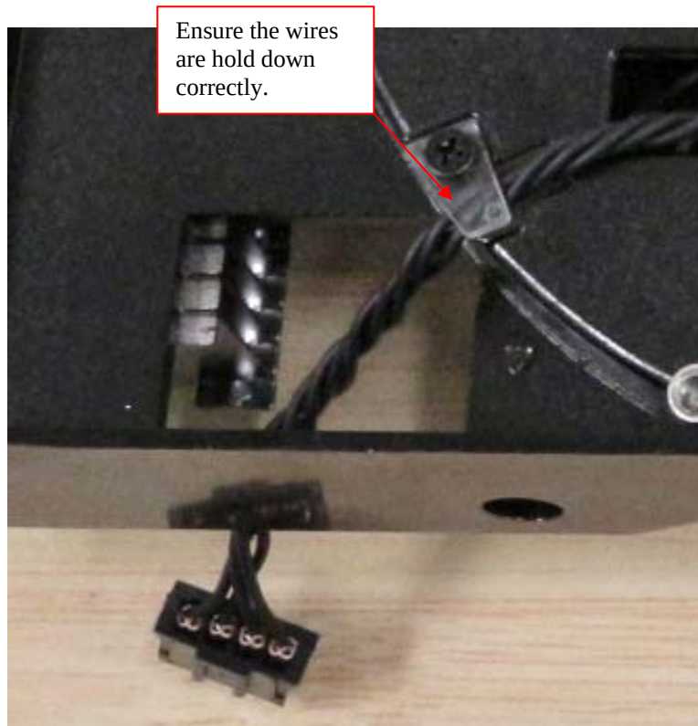
Figure 2m: Twist (approx. one full twist per centimeter) and insert fan power cable to the 4-pin header.
