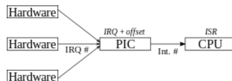
Path of an interrupt, from hardware to CPU
